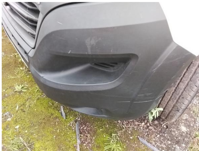
2: Bumper Front Scratched Over 100mm Thru Paint
