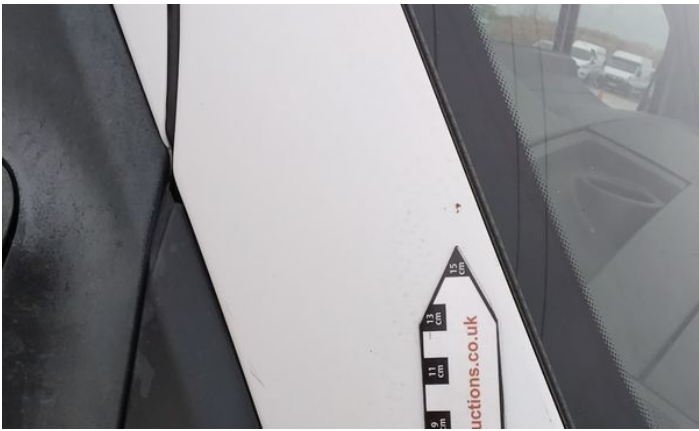
9: Door osf Scratched Over 25mm Thru Paint
